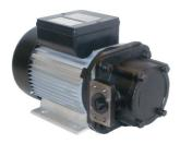
For lubricating oils. Without accessories. Self-priming gear pump, with protection class IP55 and by-pass valve. Suitable to transfer lubricating oils. Recommended for system with 10 bar maximum pressure.
